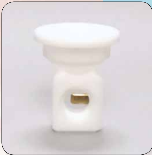
Pictured above is the unique Microtrac Zeta Cell, which is removable and easy to clean.
