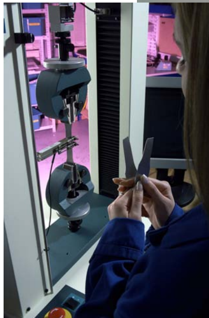
Fig2. Dumbbell specimens of sheet steel being tested on an H75kS.
