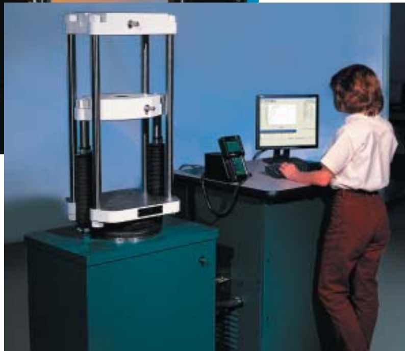
Fig. 2. Typical 60,000 lbf (300 kN) Super "L" with handheld controller and optional computer system.
