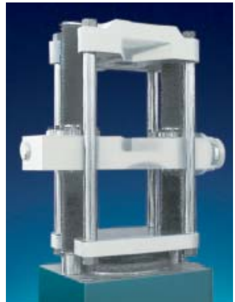
Fig. 8. Typical 400,000 lbf (2,000 kN) standard Super "L" load frame with semi-open front crossheads.
