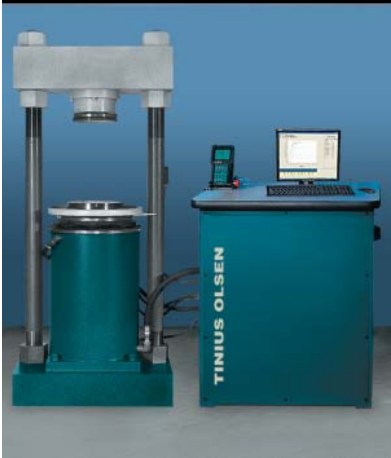
Fig. 1. 400,000 lbf (2,000kN) capacity compression only Super L with optional computer control.
