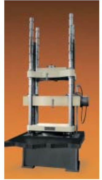
Fig. 3. Typical 400,000 lbf (2,000 kN) Deluxe Super "L" load frame with a high base (can be arranged for floor or pit mounting).
